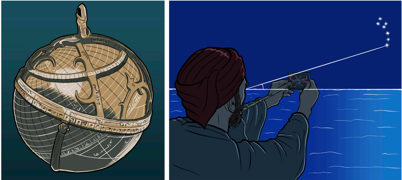
Astrolabes (left) are pretty complex instruments that help sailors determine latitude using stars. But not all technologies had to be complex. The kamal (right) was basically just a board with a knotted string that was held in the teeth and lined up with the North Star to determine latitude. OER Project.
